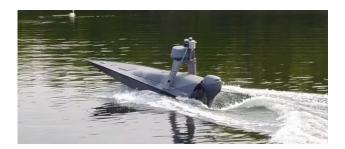
Fig. 1. Piraya autonomous unmanned surface vehicle
