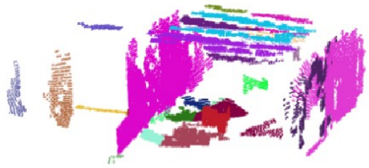
(f) Failed alignment of scans 19-20- Visualization using planar segments
